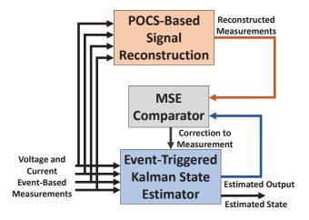
Fig. 1. Structure of the proposed event-based optimal state estimator.
