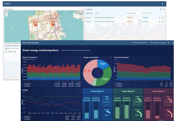
Fig. 4. Developed web-based dashboard using the Thingsboard IoT platform.
