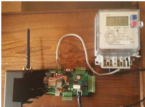
Fig. 3. Developed IoT-centric hardware prototype with the connected smart meter over the RS-485 protocol.
